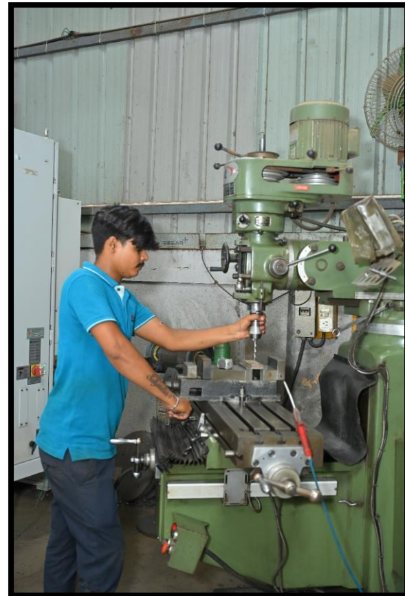
Machine 3- M1TR Machine Travel Size-X- 950 Y-360 Z-300
