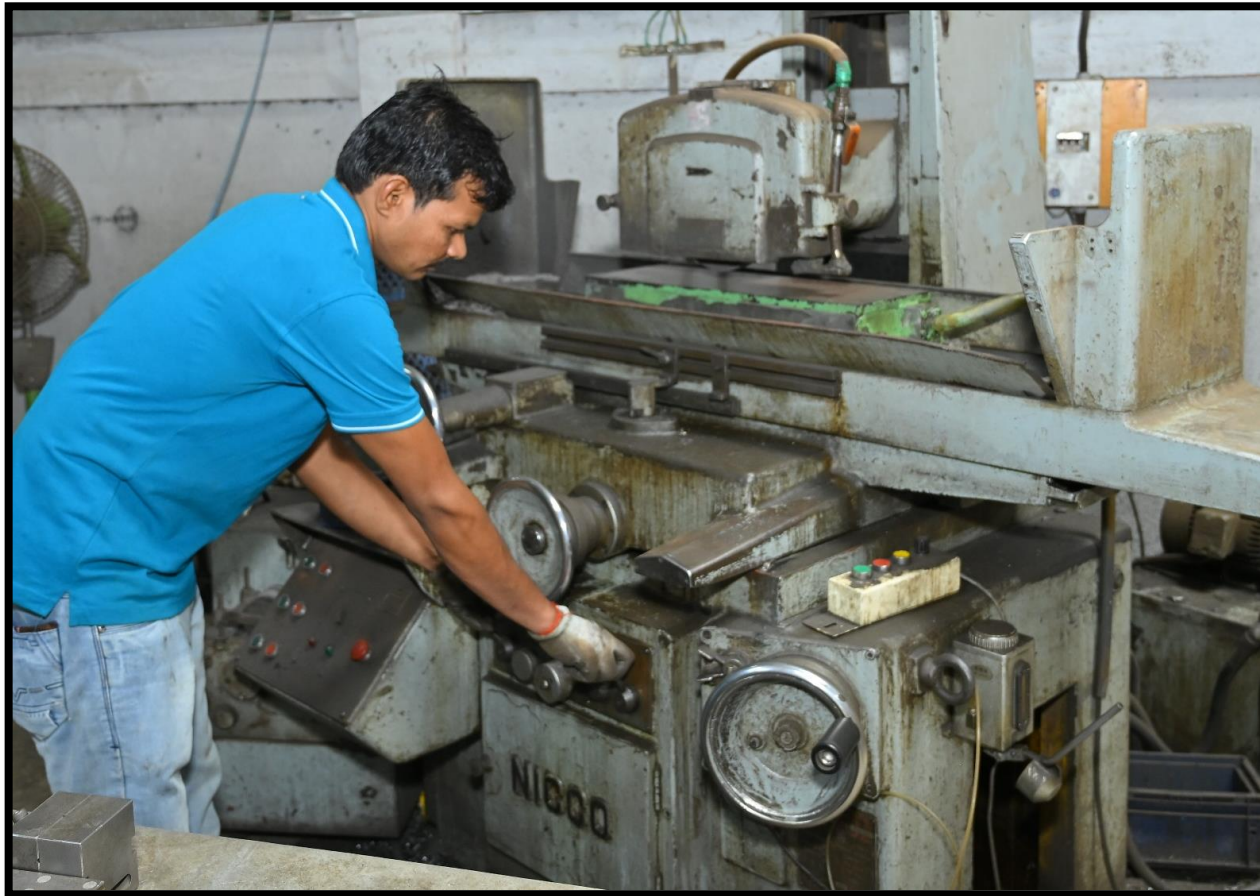
Machine 5- Surface Grinding Machine Machine Travel Size- X- 400 MM Y-250MM
